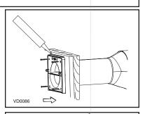
**4.** Snap the assembled exterior hood on its backplate and secure with 2 provided screws (#8 x 3/4" long).
